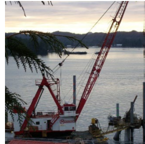
DERRICK 8 Capacity 60 Tons
