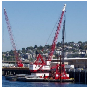
DERRICK 3 & 6 Capacity 50 Tons
