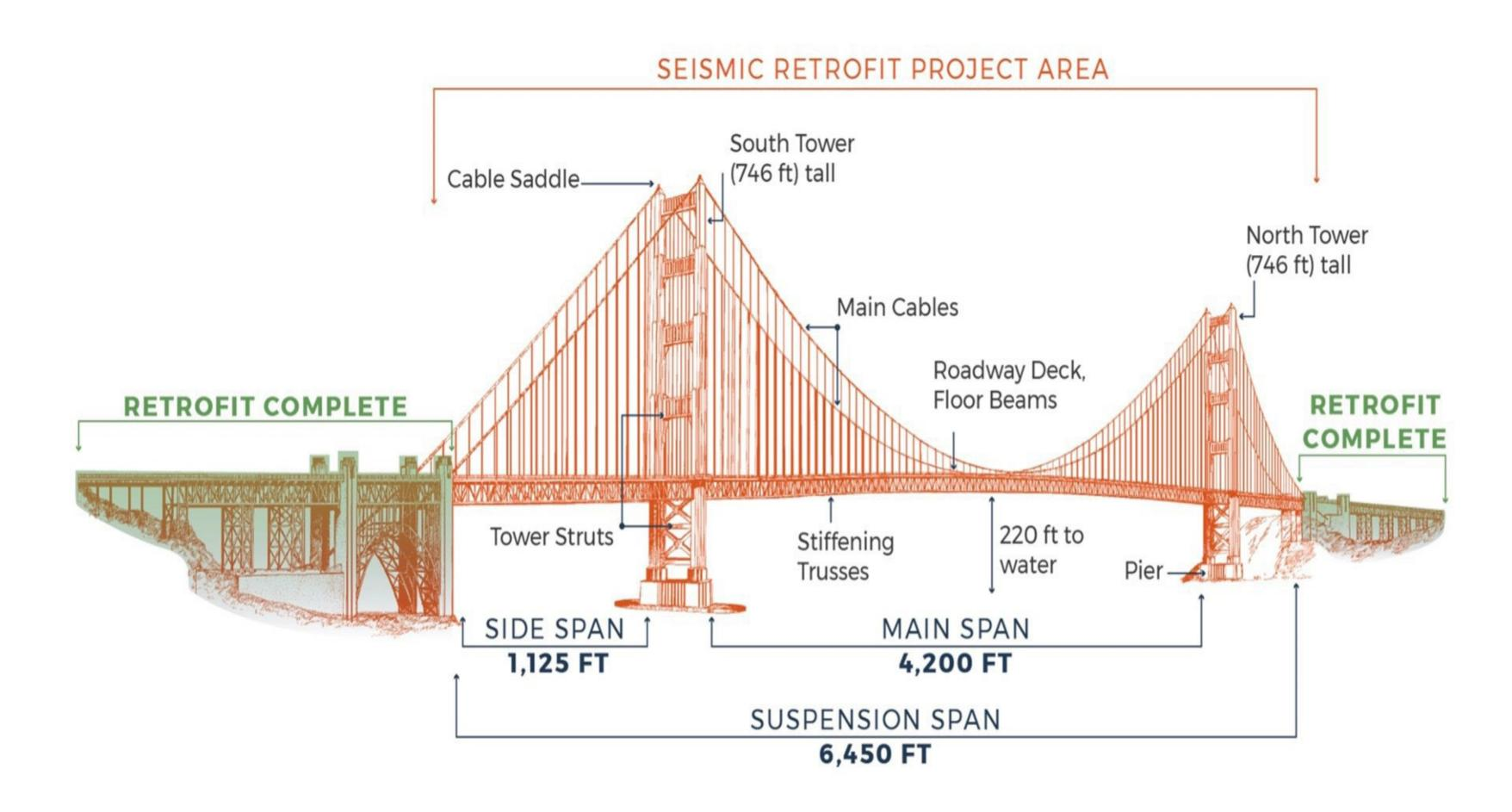
The Golden Gate Bridge can safely withstand a large earthquake today, but it could sustain significant damage that would require the Bridge to close for an extended period - or even need to be replaced altogether. The final phase of the Seismic Retrofit Project will enable the Bridge to remain operational after a major earthquake. The project will also repaint the South Tower.
