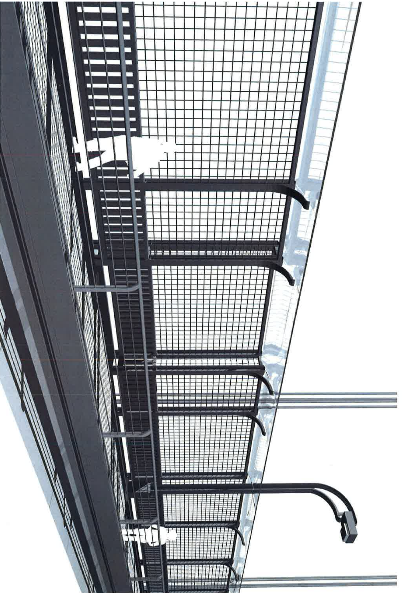
FIGURE 1.4a - EXAMPLE OF CONCEPT 1 (EXAMPLE SHOWN WITH HEIGHT OF 14'-0" TRANSPARENT WINGLET OF 64", VERTICAL AND HORIZONTAL WIRE MESH OF 6", SOLD RATIO OF 11%) VIEW FROM ROADWAY
