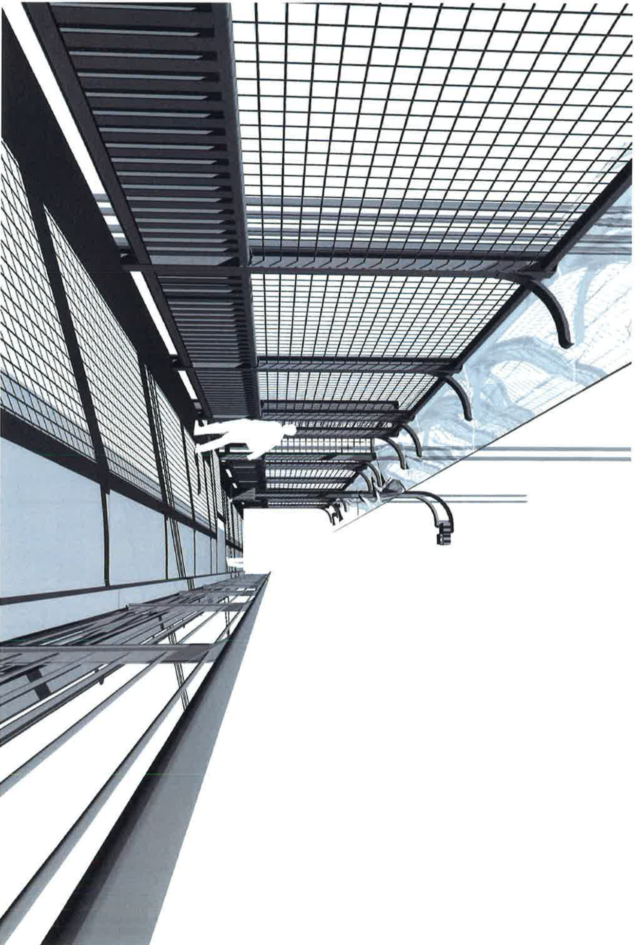
FIGURE 1.4b - EXAMPLE OF CONCEPT 1 (EXAMPLE SHOWN WITH HEIGHT OF 14'-0" TRANSPARENT WINGLET OF 64", VERTICAL AND HORIZONTAL WIRE MESH OF 6", SOLID RATIO OF 11%) VIEW FROM SIDEWALK
