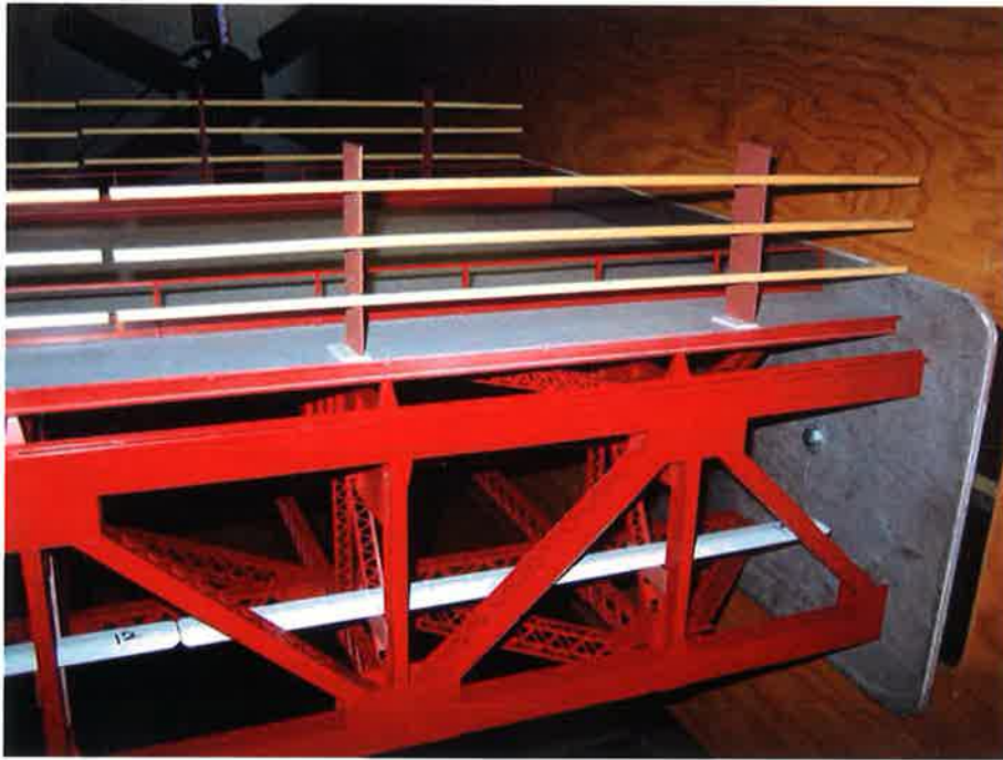
Vertical 12' barrier with below deck winglets/catwalks (Test number W1)
