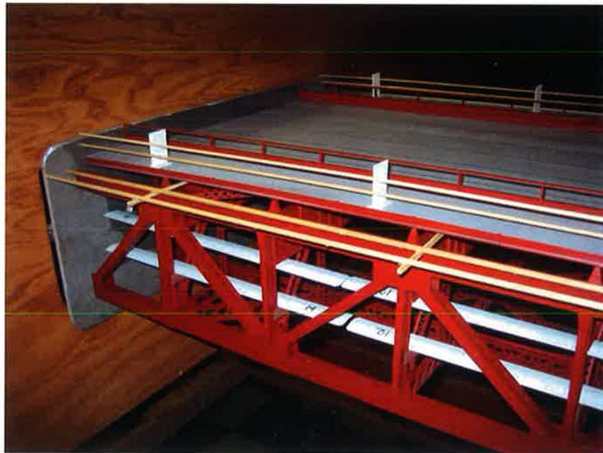
Horizontally projecting 10' barrier with a modified pedestrian railing and with below deck winglets/catwalks (Test number W6)
