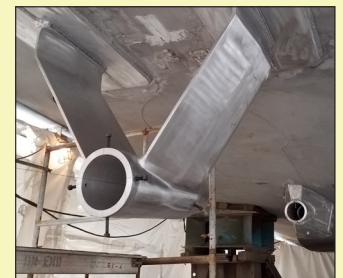
The strut and stern tube were custom made for the M.S. Sonoma.
